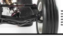
Viewing the Spyder head on reveals the arms' gullwing shape. It's easy to visualize how straight arms would require the shocks to sit higher relative to the chassis.
